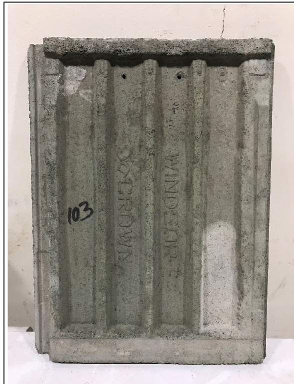
Photo No. 3 Impact Tile, Rear View
